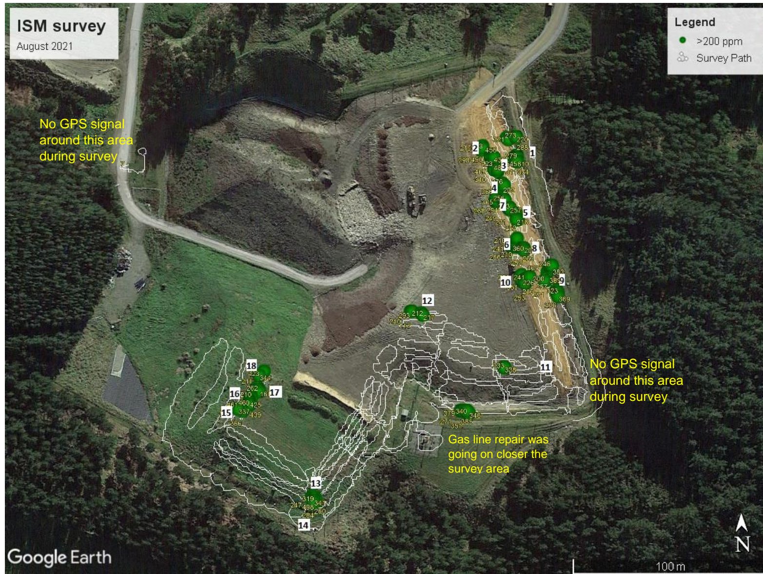
Figure 1: Map showing Levin Landfill surface emissions survey 10 th August 2021, areas in Green >200ppm.
