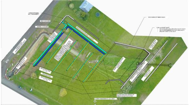
In low flows, stormwater travels through the first stage of the detention area in a zig-zag manner to maximise travel time; this area will be planted with wetland type species to treat stormwater. Planting plan is to be confirmed with iwi and Horizons. The embankment includes a low-level culvert to ensure low flows can continue to flow downstream.
