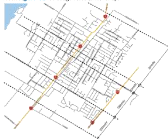
Figure G1. Design soakage rates for stormwater soak pits associated with infill developments up to 12 units in Levin.
