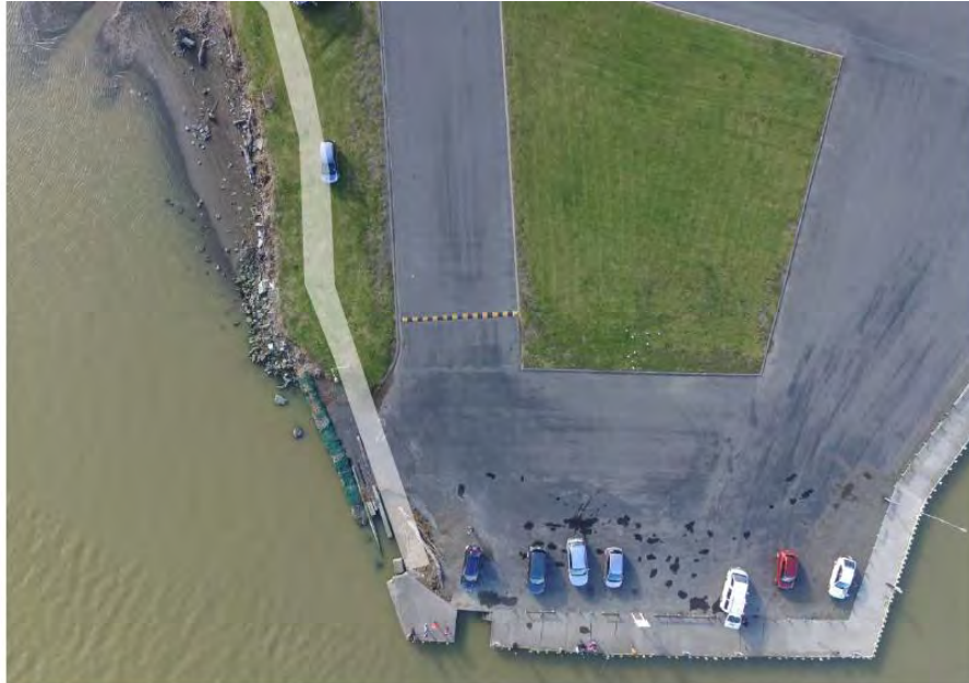
Figure 1 - Erosion behind damaged gabion basket seawall at south western corner of Foxton Wharf and indicative footpath extension alignment
