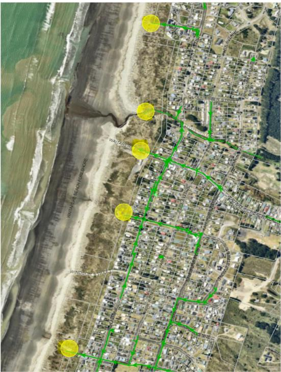
Figure 2: Waitārere Beach Stormwater Discharge Locations
