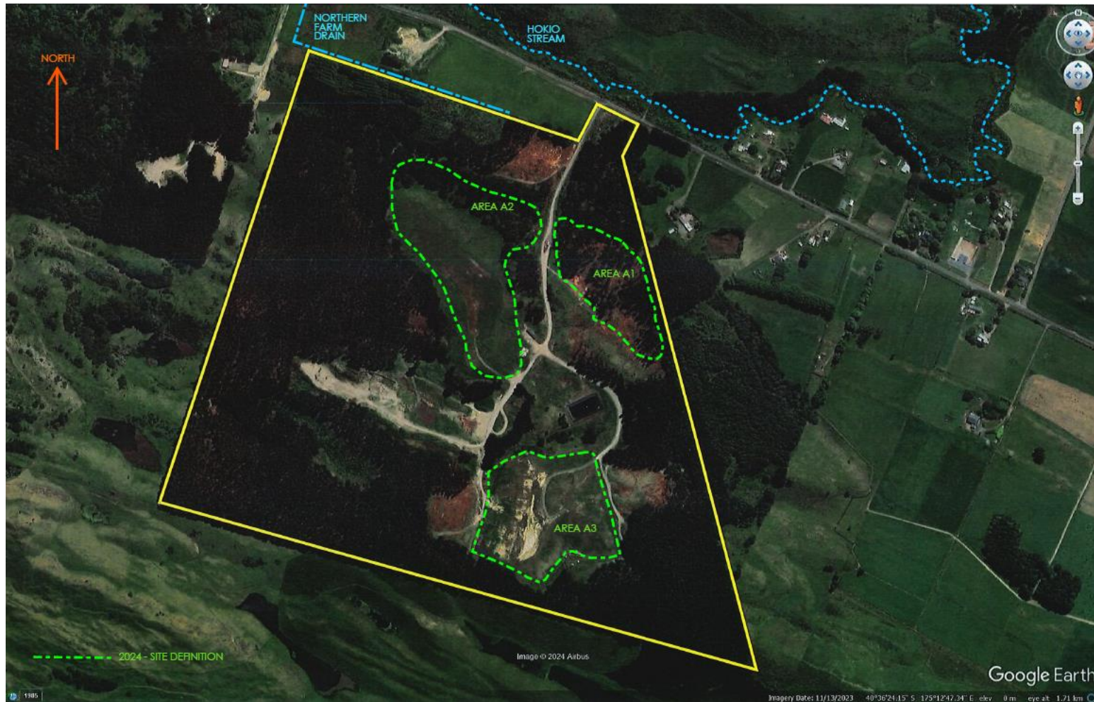
Figure A- 5: Definition of closed landfill areas used within this CLMP (source: Google Earth).
