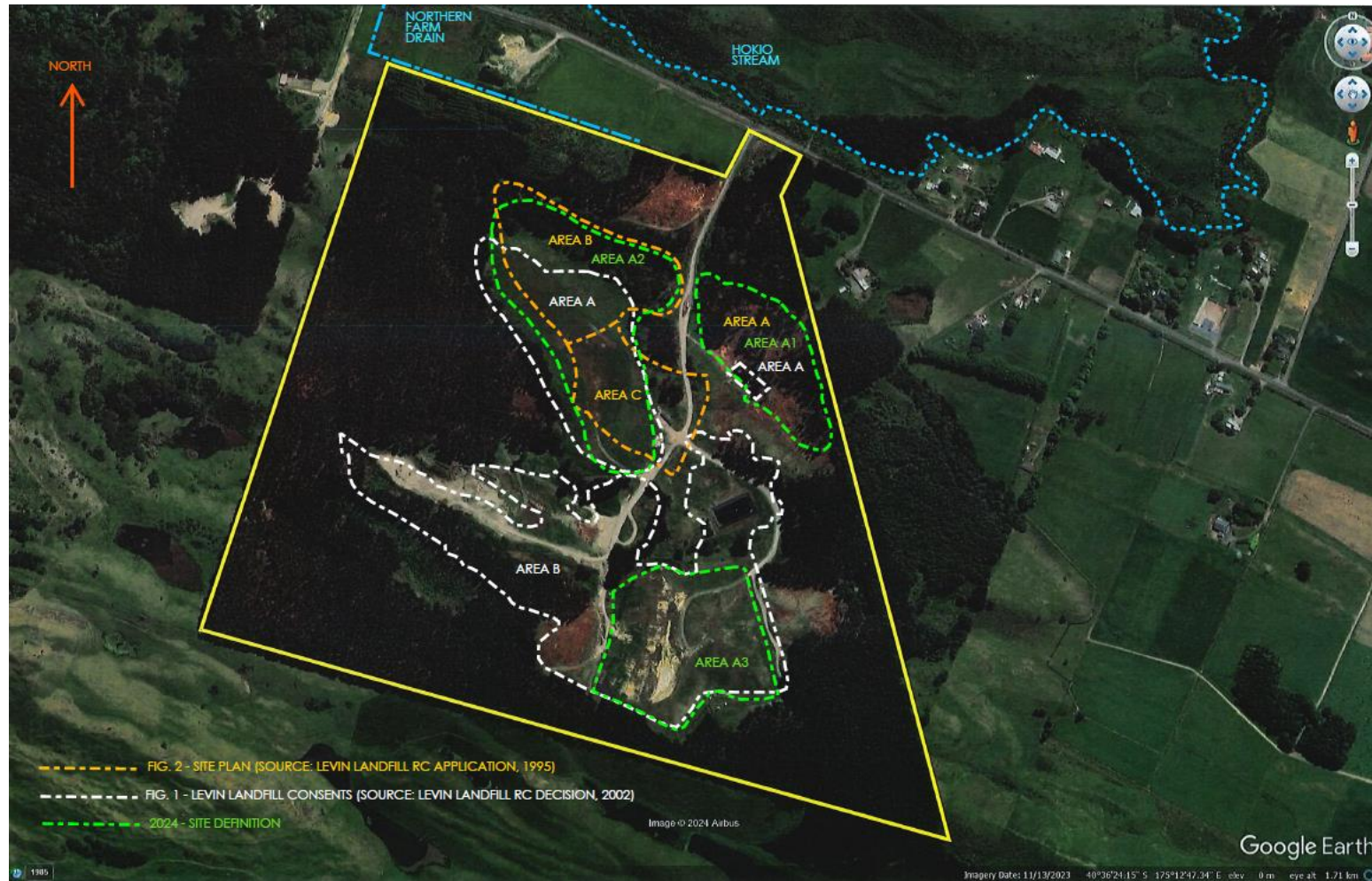
Figure A- 4: Delineating areas of old, unlined landfill (Areas A1 and A2), and area of new, lined landfill (Area A3). Note, extents of areas are approximate (source: Google Earth).
