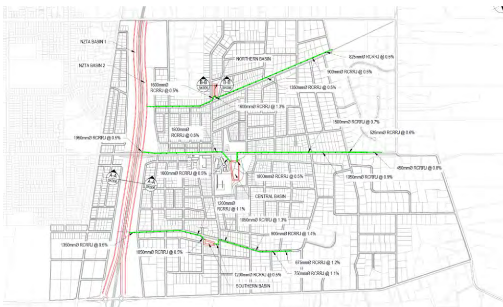
Figure 2 Excerpt figures from Stormwater Management Plan showing post-development drainage catchments (top) and overall trunk reticulation servicing layout (bottom)
