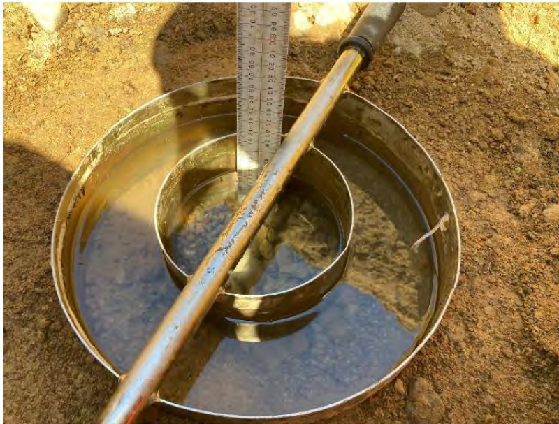
Figure 4 Double Ring Infiltrometer setup used for soakage testing
