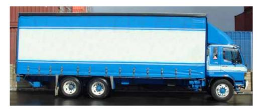
Rigid trucks up to 12.6 metres are also possible, however, with these not being able to tow a trailer, they tend to be designed for special purposes (eg furniture removal or as transporters for light contracting equipment such as rollers). Should a specific design anticipate the presence of these longer trucks, the tour coach tracking curve should be used to represent the 12.6 metre long rigid truck.
