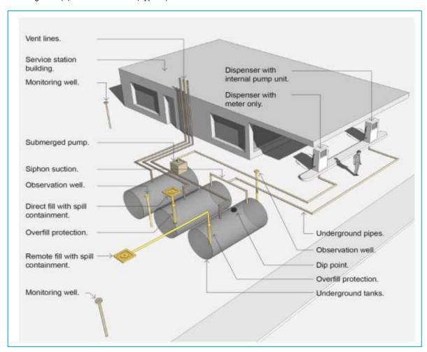
Fig 10.9 (1) Tank Installation (Typical)
