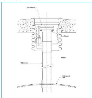
Fig 11.6 (b) Over Fill Device (Typical)
