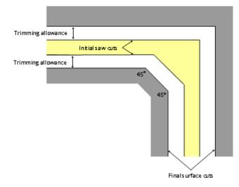
Figure 1-6 is an example of how an irregular excavation should be expanded to form a more regular shape to minimise disruption to the surface.
