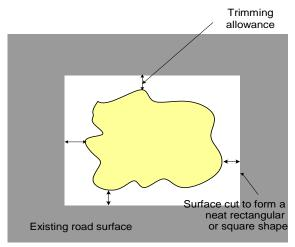
Figure 1-6: Finishing of irregular shaped excavations
