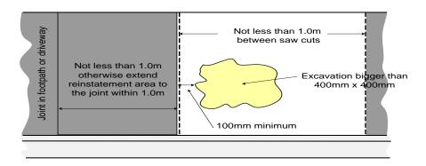
Figure 1-9: Reinstatement of concrete path or driveway
