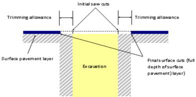
Figure 1-3: Standard trimming for Trench cuts
