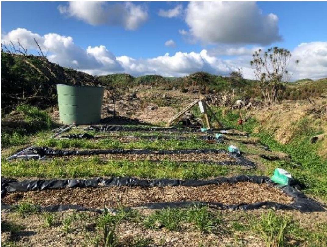
Four small scale bio-reactor installations at the POT for research experimental purpose.
