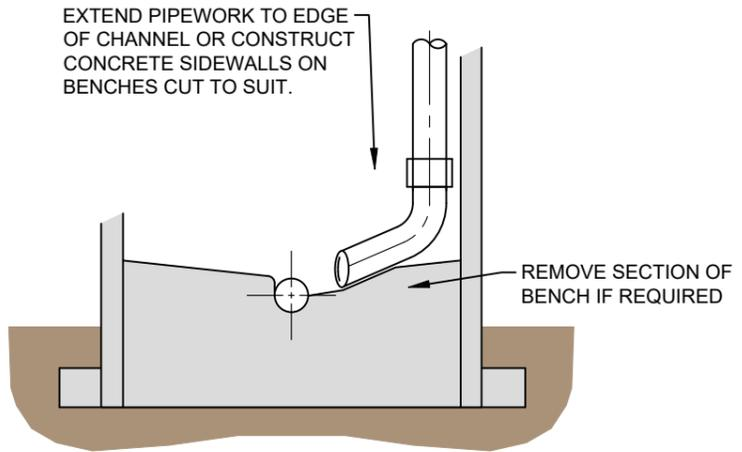
**INTERNAL DROP - POST CONSTRUCTION INSTALLATION DETAIL**
