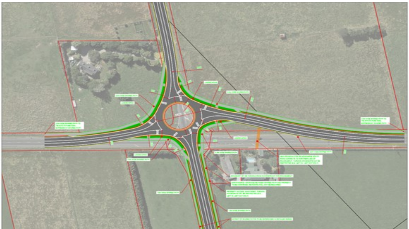
Indicative roundabout layout Tararua Road/ SH57
