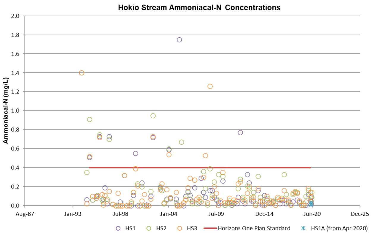
Figure 5-3: Ammoniacal-Nitrogen Concentrations measured in Hokio Stream, since 1994
