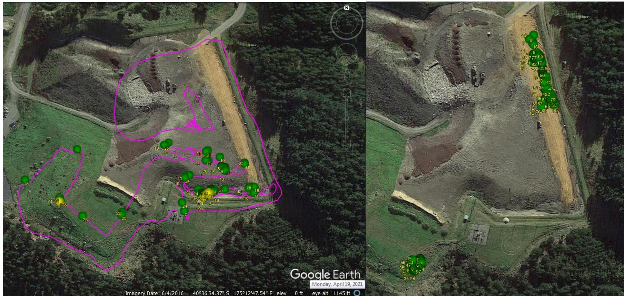
Figure 5: Surface emission readings after remediation works. No areas above 200ppm, Yellow>50ppm, Green 0-50ppm.
