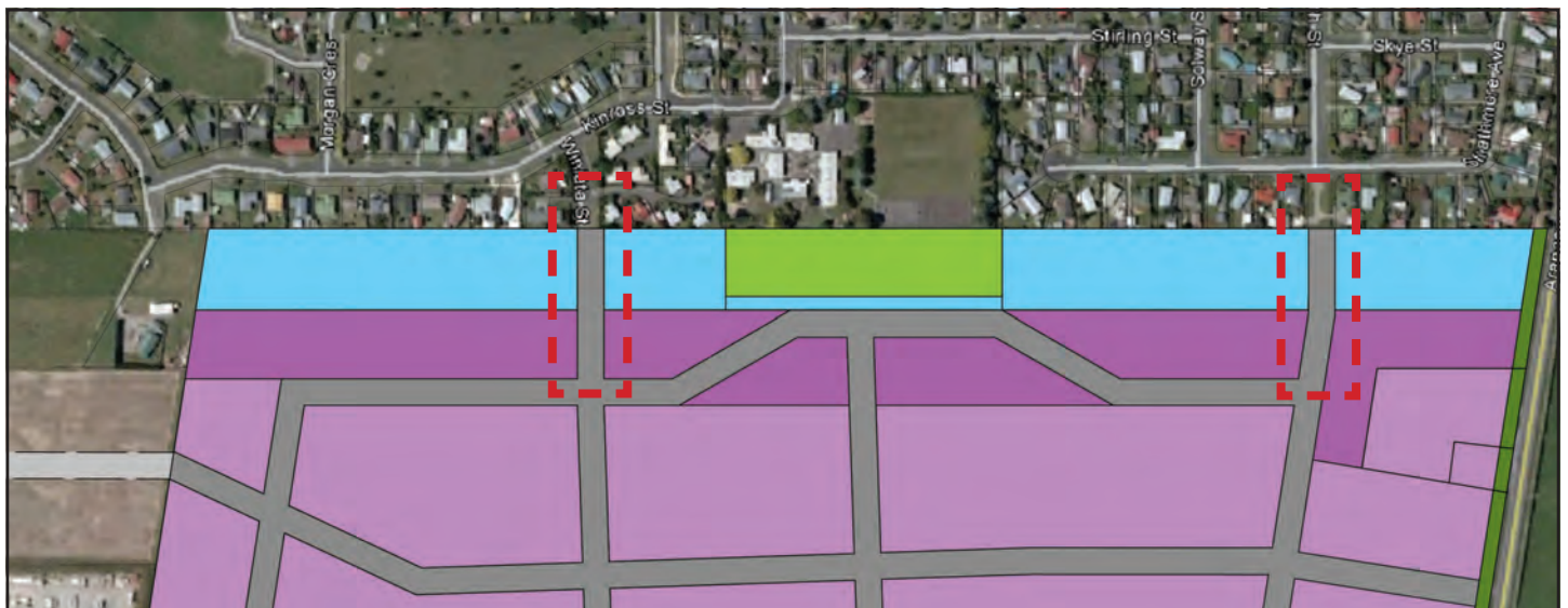
Figure 10. Internal access roads connecting to existing residential area
