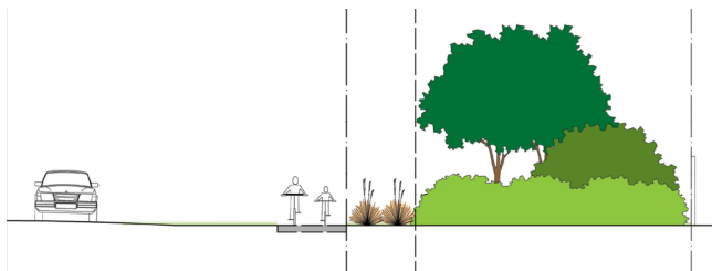
5. Hierarchy of vegetation heights to provide screening and natural surveillance
