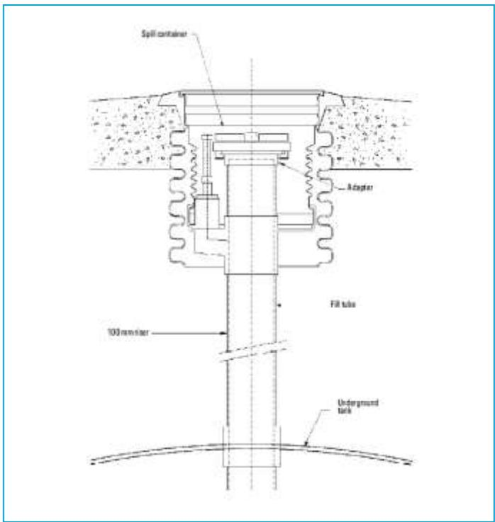
Fig 11.6 (b) Over Fill Device (Typical)
