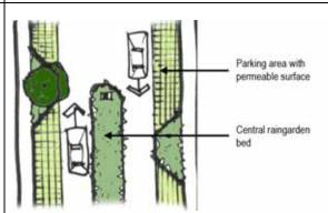
An example diagram of a street type which reduces pavement impermeable surface and manages stormwater runoff through percolation into the ground (rather than piping it away). This type of approach will work where the ground conditions are suitable, but will not where for example the groundwater is at a high level.
