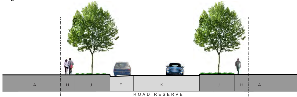
Urban Local - Option 2 (for high volume parking areas) 9.5m Carriageway, inc. parking to one side
