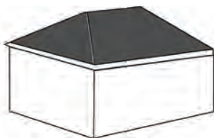
Typical roof types: Hipped roof
