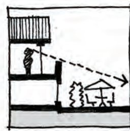
Screen with balcony balustrade
