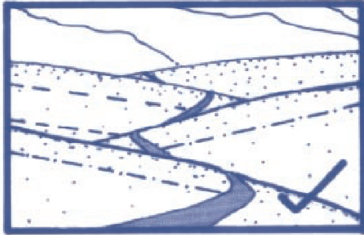
Figure 18: Roads that follow contours are responsive to the shape of the land and are less obtrusive.
